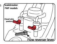
lower connection of the heat exchanger, and this flow direction should be maintained in this direction for the duration of the descale.
